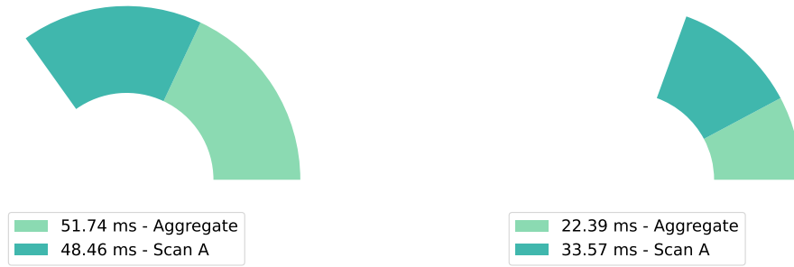
(a) Columns a and b located on the same DDR-SDRAM Node. (b) Column a located in DDR-SDRAM and b in HBM.
